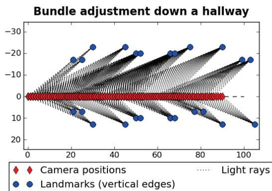
**Figure 2. Camera path, landmarks and detections in a visual SLAM problem. The lines related to each detection meet at the landmarks. Figure reproduced from [17].**
